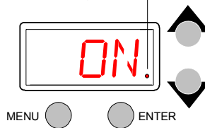
Figure 4-2. A dot always appears in the LED display whenever preset playback is on.
